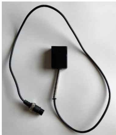
Figure 10. The IR motion sensor used for this this experiment.
