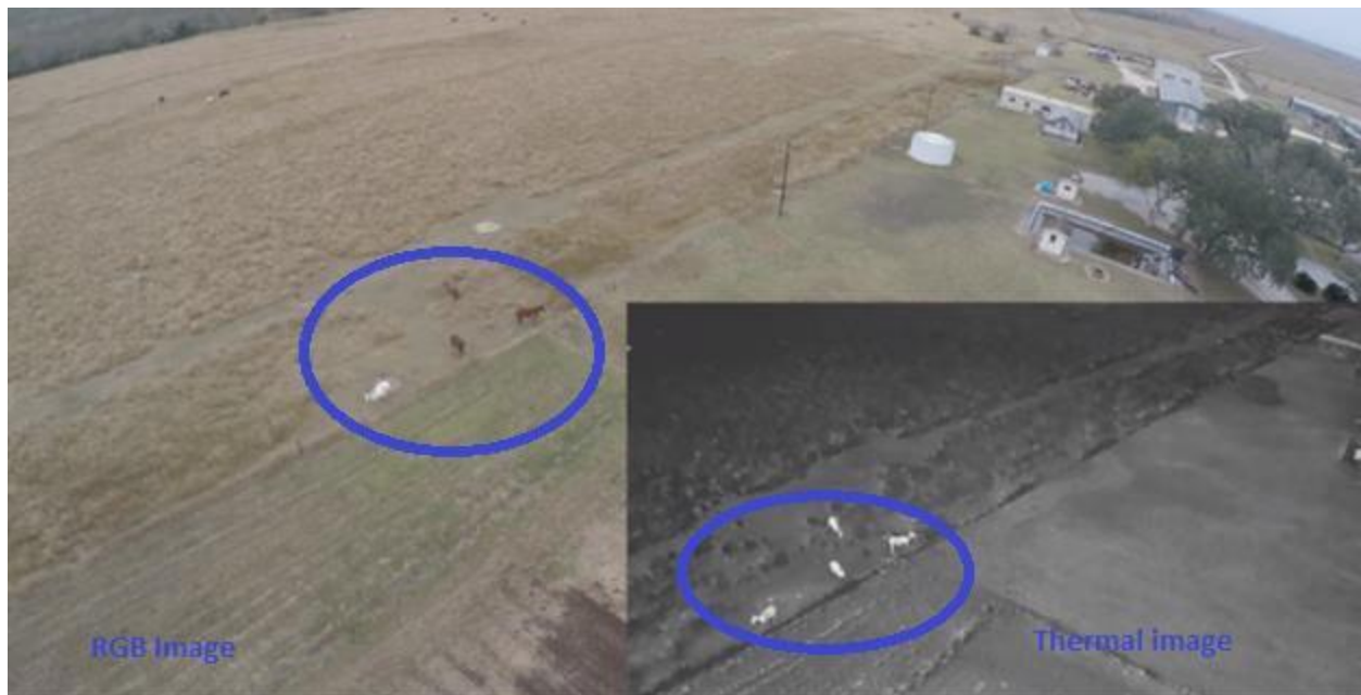
Figure 9: The RGB and Thermal images from the drone. The cattle are easier to detect in thermal images.
