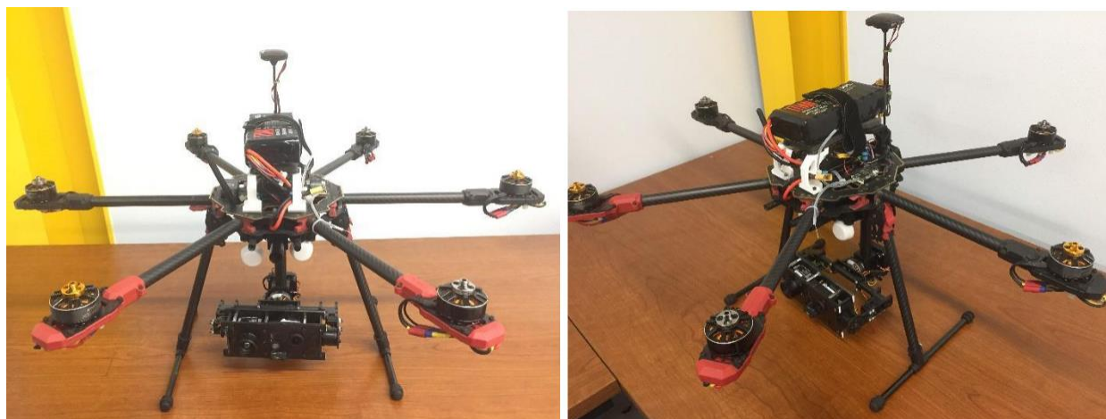
Figure 1. Images of the Hexacopter set up. Six-motors set up for maximum redundancy and payload.
