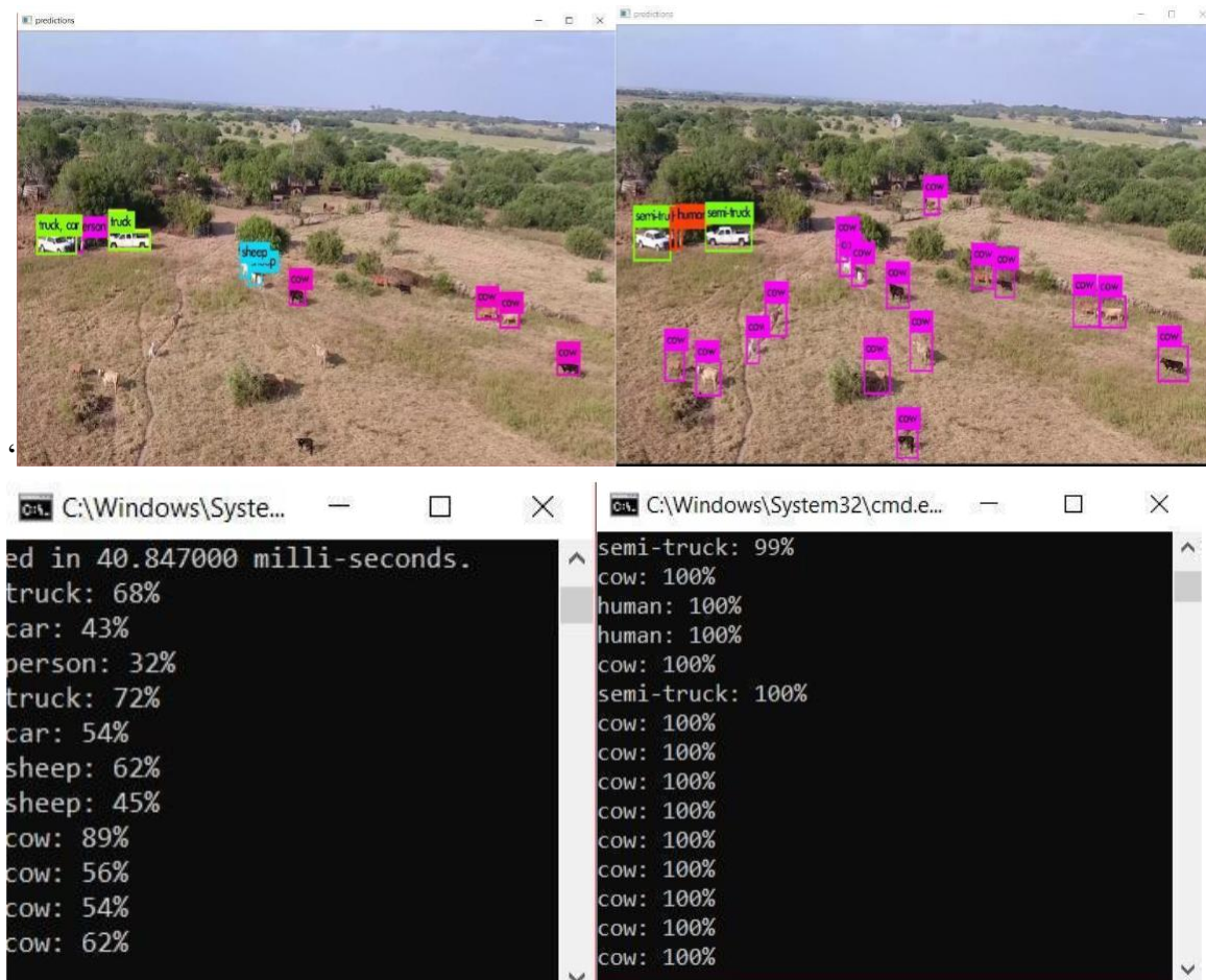
Figure 9. The result generates with “YOLO” algorithm before (left-Yolov3) and after(right). Top left figure: YOLOv3 could not detect all the objects in the scene, some classification is not correct. Bottom left figure: The confidence level of detected object for YOLOV3.Top Right figure: The result from our custom training data. Bottom right figure: The confidence level of detecting the right object for our custom training data.
