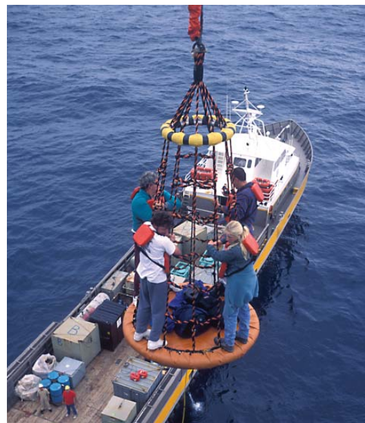
Figure 13. Team offloading from the M/V Norman McCall to the platform via a Billy Pugh personnel basket.
